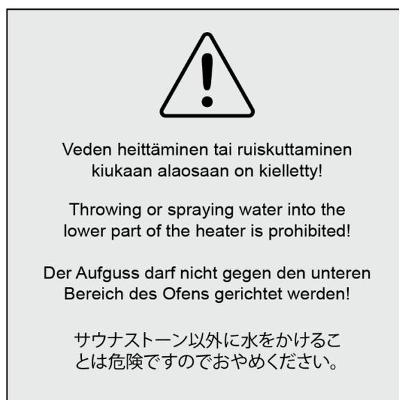
The warning sticker that came along the heater delivery is recommended to be glued to the bottom side of the heater or to another visible place in the sauna.
