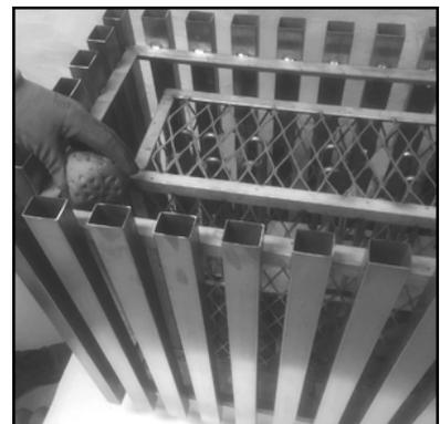
9. Set the stones (large and small Kerkes tetra stones) between the inner and outer frame. At last set the stones on top of the inner frame and the coverpart/lid.
