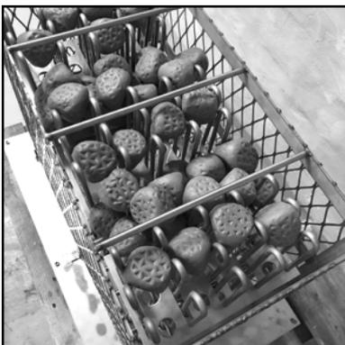
7. Insert the top part element guides so that they lean against the horizontal steel pillars. Place appx. 25-40pcs small KERKES ceramic stones between the elements depending on the model. That way we can avoid the elements to bend against each other.
